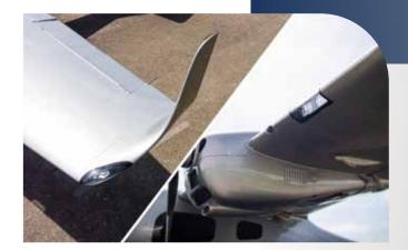
The new wing position / anticollision lights are integrated into the winglets and now equipped with state-of-the-art LED technology. This not only enhances efficiency, style, and visibility but also offers a more eco-friendly and durable lighting solution.
